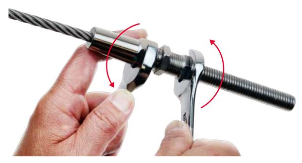
Use 2 proper size wrenches, one on the housing and the other one on the head of the fitting and starts to tighten in opposite direction as far as possible.
